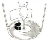
**6.** Retain plate by screwing the crosshead screw with washer trigger attached into the retaining bush after first observing the following **IMPORTANT CHECK**.
