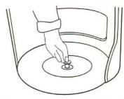
Locate screw and washer together into central spacer.
