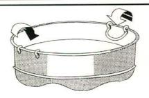
NB Ensure that the liner handles are turned fully inwards after the liner has been emptied.
