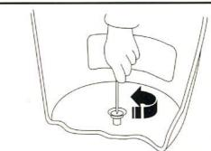
2. Using a screw driver, unscrew the panhead screw and thermoplastic washer (which will now be deformed) from the central spacer. Remove and discard the deformed thermoplastic trigger washer from the panhead screw.
