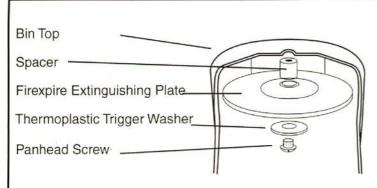
1. After first ensuring the Firexpire plate is cool and the contents of the liner compartment have been extinguished, remove the top section of the litter bin and turn the hood upside down.
