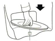
**4.** Locate extinguishing plate into position over the spacer ensuring the plate is the correct way up.
